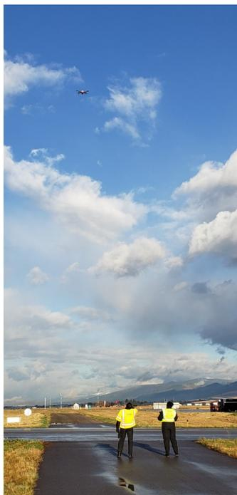
**Ground personnel from the firm Silent Falcon fly their drone over the airport’s Runway 12/30. The aircraft’s software yields data used in evaluating the condition of runway pavement.**
