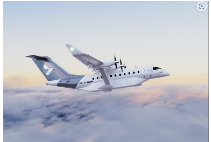
A rendering of Heart Aerospace's new 30-seat electric turboprop plane, the ES-30.
