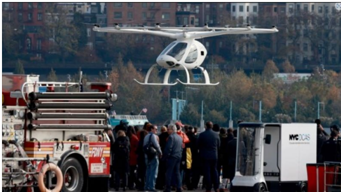
The Volocopter 2X electric air taxi takes off from the Downtown Manhattan Heliport for a test run along the East River on Nov. 13.
